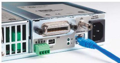
FIGURE 1. Instruments with multiple types of interfaces can help smooth the transition to hybrid systems employing LXI. Courtesy of Agilent Technologies.
